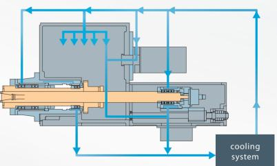
■ The spindle cooling system uses oil cooling and water jacket device to give the right amount of coolant to all the bearings, motors, gears inside the spindle box. This effectively reduces spindle thermal distortion and ensures working accuracy.
