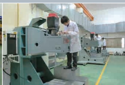
■ Gear box run-in test
