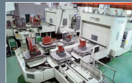
■ Japan-made MITSUI SEIKI horizontal machining center
