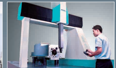
■ German-made WENZEL 3D coordinate measuring machine
