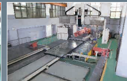
■ Japan-made TOSHIBA bridge type 5-face machining center
