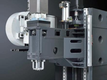
Adopted with high power HEIDENHAIN spindle motor, 12,000 rpm and 15,000 rpm spindle for options to meet your variety of processing characteristics.
