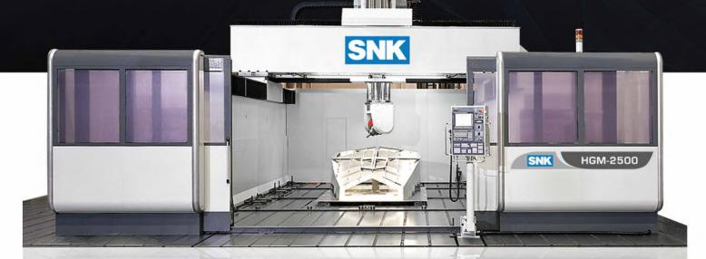
The **HGM Series** of 5-Axis High Rail Gantry Profilers from SNK is the perfect choice for the machining of complex, multi-faceted large parts. The combination of high speed and high power, together with 5-Axis simultaneous contouring capability, make them ideal for the aerospace, transportation and die/mold industries. Extraordinary rapid feedrates of up to 2,400 ipm on the X and Y axes, 7,200 deg/min feeds on the
