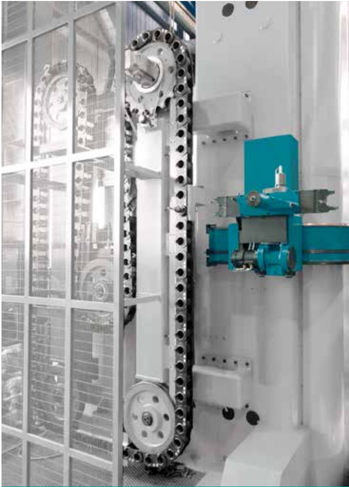
chain type tool magazines, column side mounted, with capacity from 80 to 120 tools
