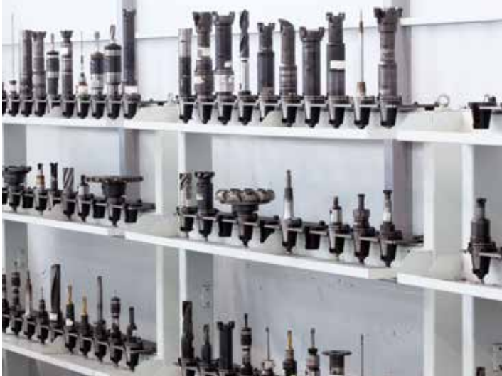
modular rack type tool magazines, floor mounted, featuring large capacity and limited floor space
