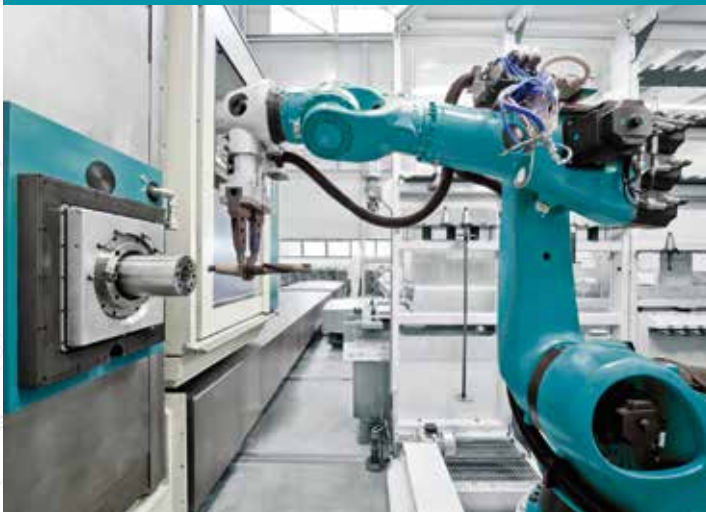
rack type tool magazines, floor mounted and served by robot, with capacity up to 1000 tools
