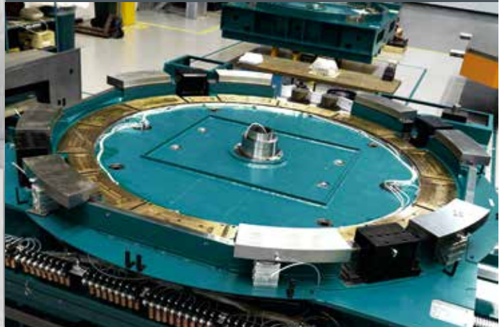
hydrostatic thrust bearing and hydrostatic pads
