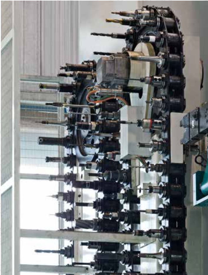
chain type tool magazines, column side mounted, with capacity from 60 to 140 tools
