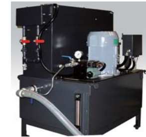
High pressure coolant unit
