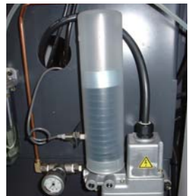
Automatic grease lubrication unit for linear guides and ball screws [Opt]
