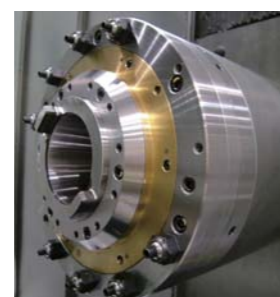
Spindle for Dual-contact holder of BT50
