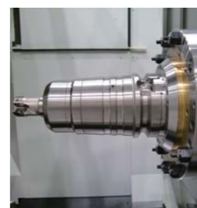
Dual-contact holder is loaded, no space between holder and spindle nose.
