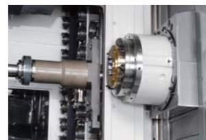
ATC arm returned to origin position
