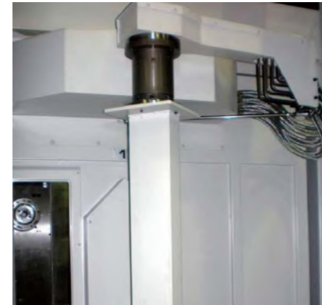
Example of the use of 6-port rotary joint (HM400/500S, HM5000/HM6300S)
