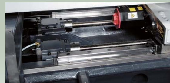
Z axis twin-ball-screw
