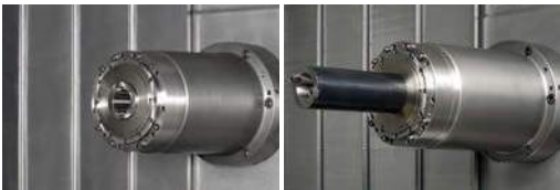
Quill spindle standard position: 0mm(0") Quill spindle extended position: 300mm(11.8")
