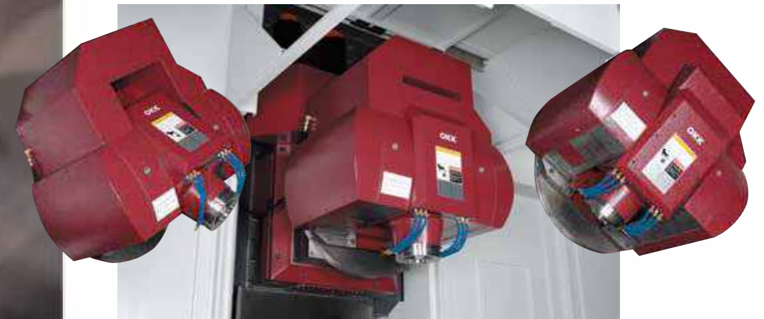
Tilting and swiveling structure of the spindle
