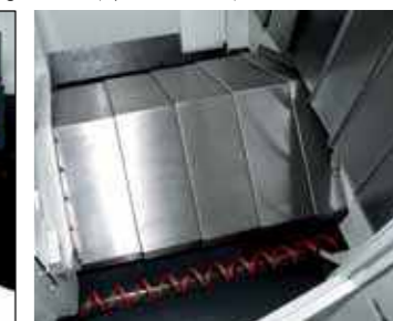
Coil type chip conveyor
