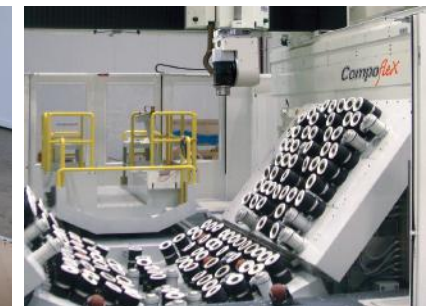
Speeder can integrate Compoflex, the universal flexible tooling system developed by Jobs that allows the reference and clamping of composite parts
