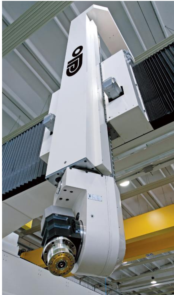
Crossbeam structure optimised for ensuring the necessary accuracy and stiffness even with the completely extended ram
