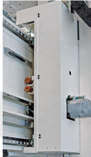
Cross axis frame (Y axis) composed of an electrowelded steel crossbeam with two preloaded roller guide-ways for Y-axis saddle movement
