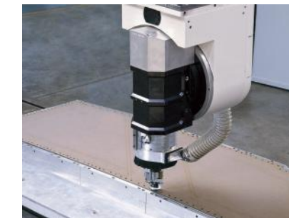
A suction system, developed by Jobs, equipped with programmable mobile hood can be integrated on these heads. This solution allows the maximum dust suction efficiency over the entire work area of the machine
