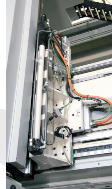
Transversal axis frame (Y axis) composed of a dully optimized crossbeam with wide-section guides and preloaded rollers for saddle movement
