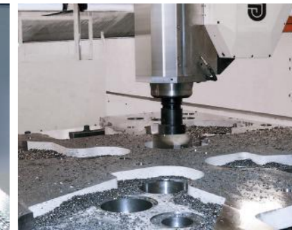
Indexed TMX head for general precision engineering operations
