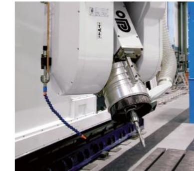
Bipolar T2D head for car design & prototyping applications
