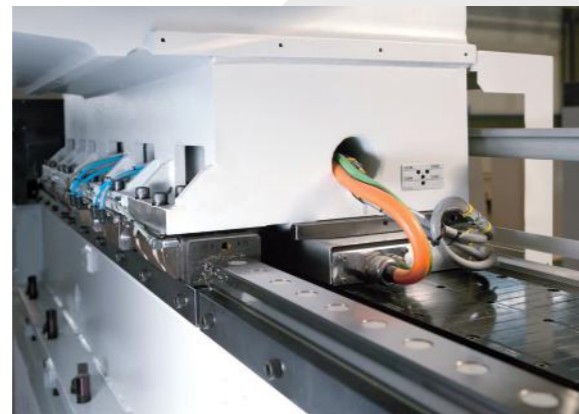
Vertical axis frame (Z axis) composed of a ram sliding within the saddle on wide-section guides with preloaded rollers
