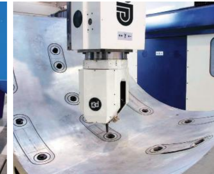
T3D Aero-configuration head for high-power machining in aerospace industry
