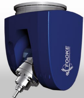
Milling head 05 High-frequency milling spindle HSK63A with 25 kW, 20,000 rpm or with 39 kW, 24,000 rpm or with 45 kW, 30,000 rpm
